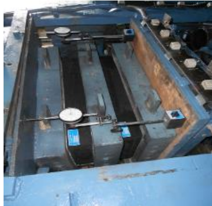
Bearing pad test
