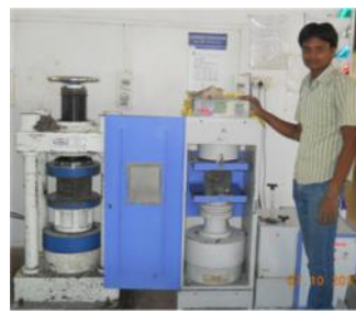
Concrete Compressive test
