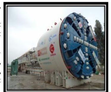
TBM prior to shipment for UAA 03 from China
