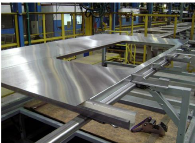
Car body- Sidewall work in progress in factory
