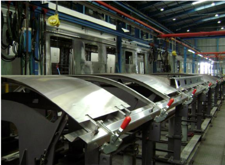
Car body - Roof structure assembly work in progress
