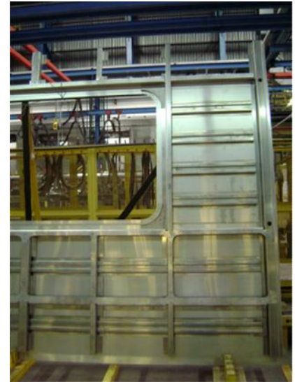
Car body -Sidewall work in progress
