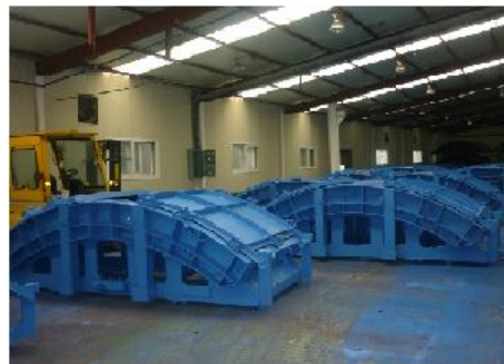
Tunnel segment moulds ready for shipment
