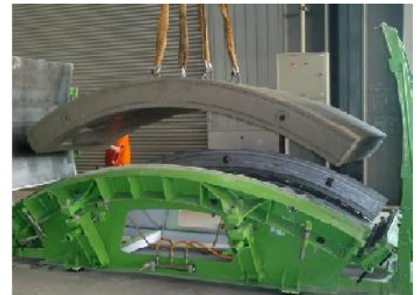
Pre-cast segment test in factory during FAT
